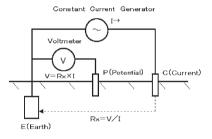
7-2 Precise Measurement (with Test Probe M-7095A)
