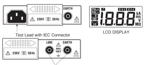
Fig. 1 Test Lead for Continuity and Insulation Testing
