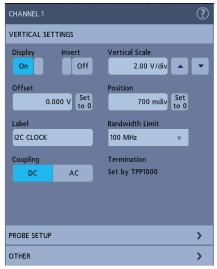
Configuration menus are accessed by simply double-tapping on the item of interest on the display. In this case, the Channel badge was double-tapped to open the channel configuration menu. Menus are dismissed by simply tapping outside of them.
