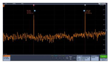
Spectral display of a bursted communication both into a device through Zigbee at 900 MHz and out of the device through Bluetooth at 2.4 GHz, captured with a single
