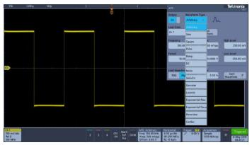
Waveform type selection in the integrated AFG.
