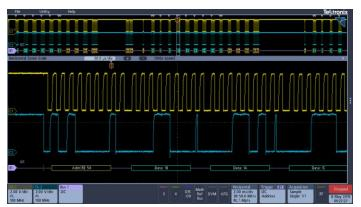
Triggering on a specific address and data packet going across an I<sup>2</sup>C bus. The yellow waveform is clock and the blue waveform is the data. A bus waveform provides decoded packet content including Start, Address, Read/Write, Data, and Stop.
